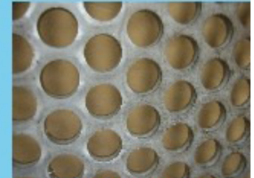
Example of perforated metal 3/16" thick. 1/2" holes, 11/16" staggered pattern 48" open area.
