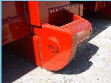
Bull Nose, Nose Rollers, Roller Finger and Axle, Grease Zerk
