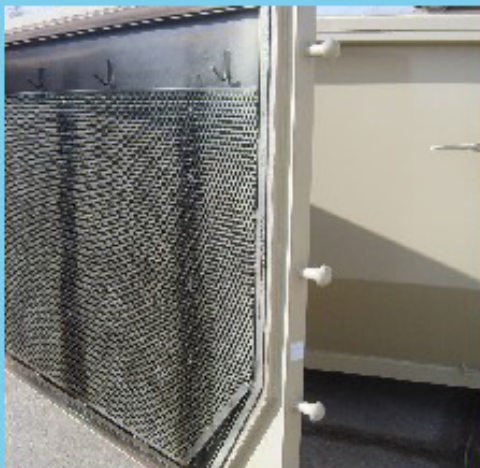
Liner hooks on door, fully gasketed rear door, knife edge seal. Stainless steel filter on door no build up.
