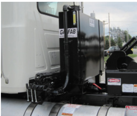
Behind the Cab Oil Tank
