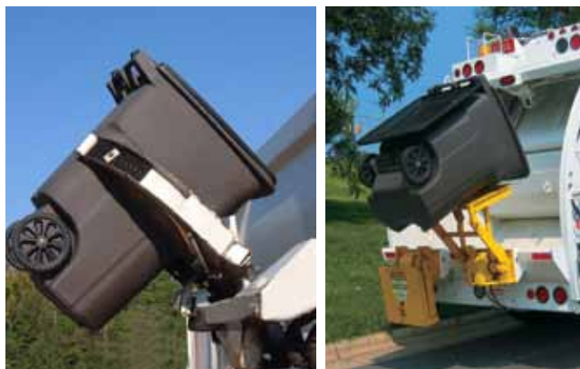
EVR II is compatible with both the fully automated arm (left) and the semi-automated lifter (right).
