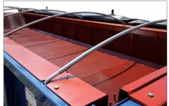
Bolt-in liners are easily removed.
